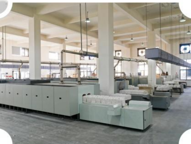
12米高温双孔逆向半自动推板电窑 12m high temperature double hole reverse semi-automatic push-plate electric kiln
